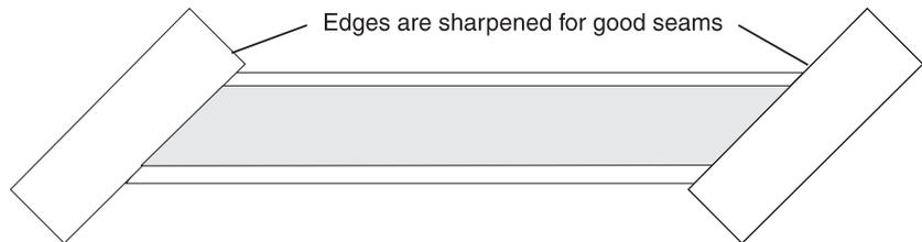
The tube is shaped by several roll stands. The last stand determines the final diameter and the roundness of the tubes. At that position there is a swimmer in the inside of the tube with two heads. The swimmer presses the wall of the tube against the last two rollers. The position of the swimmer determines the winding thickness which in small diameters correlates directly with the quality or number of cavities between the layers of the tube walls.
