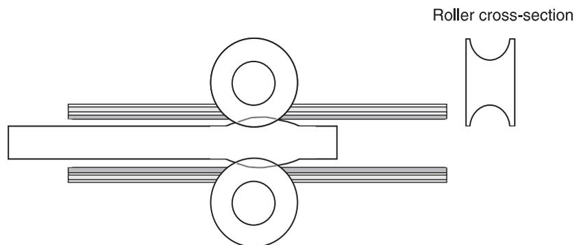
In order to compensate for the 'waviness' which can arise from the mechanical processing of the band, the speeds of the rollers are controlled so that the tube is continuously drawn. The stretching factor amounts to approx. 1.04 - 1.08.
