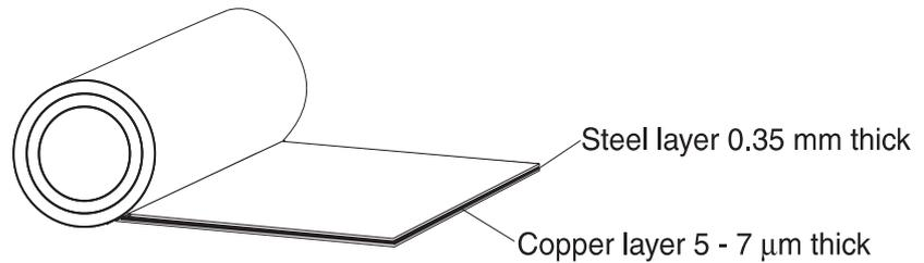
The band is cleaned in-line and oiled. The edges are sharpened with the aid of two pressure rollers in order to obtain a good internal and external seam.
