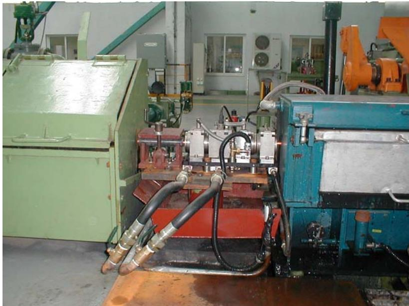
Figure 5. Water-cooled test head in the rolling mill
