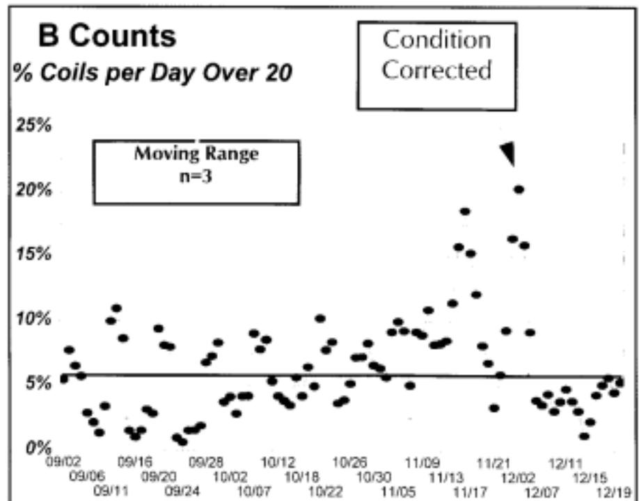
Fig. 15. Percentage of coils rolled each day whose B count exceeded 20
