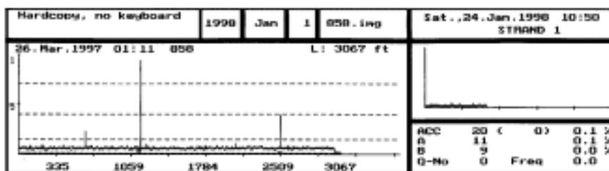
Fig. 12. Eddy current signal after guide was replaced
