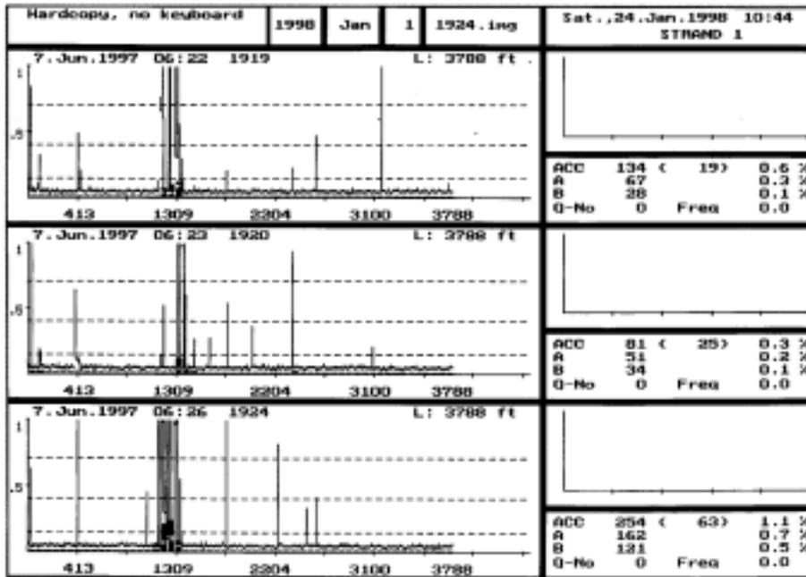
Fig. 10. Eddy current signals indicating defects induced by furnace floor refractory
