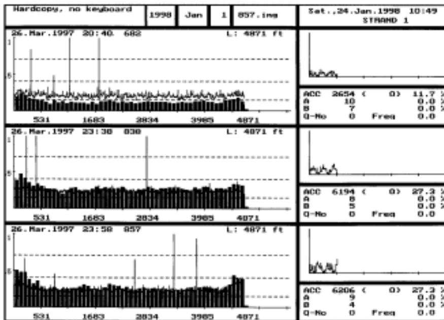
Fig. 11. Eddy current signals indicating imminent guide failure
