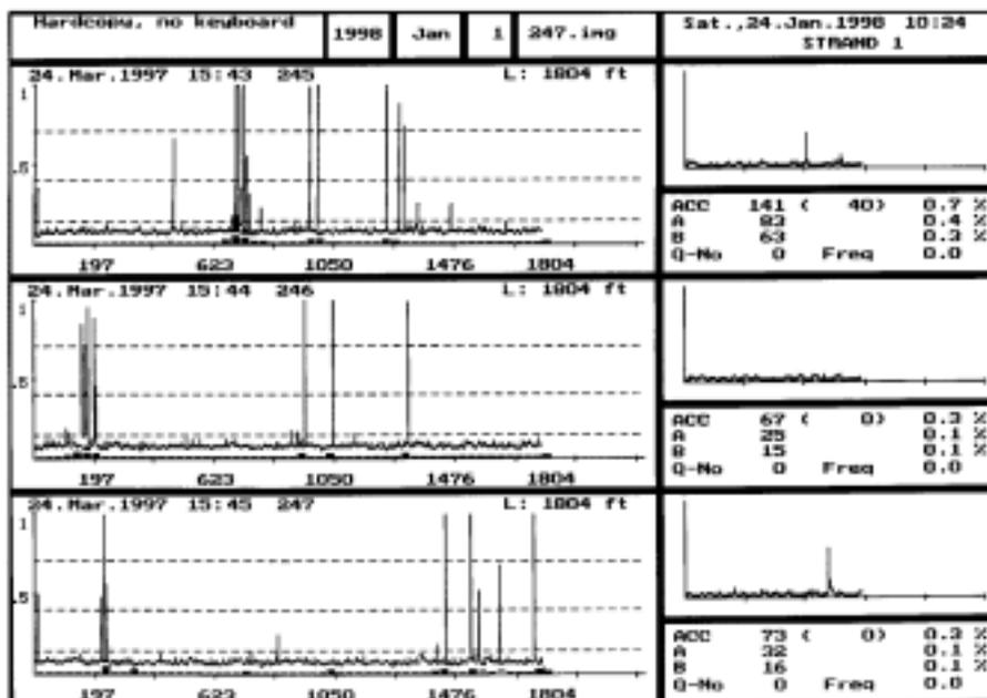
Fig. 7. Eddy current signals from billets with induced defects
