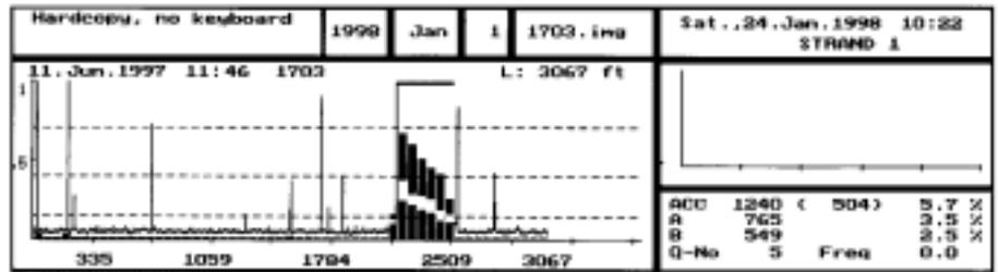
Fig. 5. Eddy current signal with vertical bars indicating multiple defects
