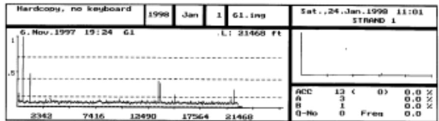
Fig. 14. Eddy current signal indicating possible seam (at center)
