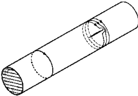
Fig. 13. Eddy current flow patterns
