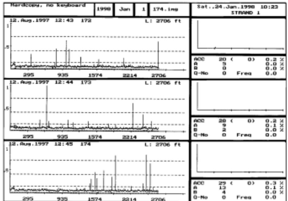
Fig. 6. Three eddy current signals in different panes
