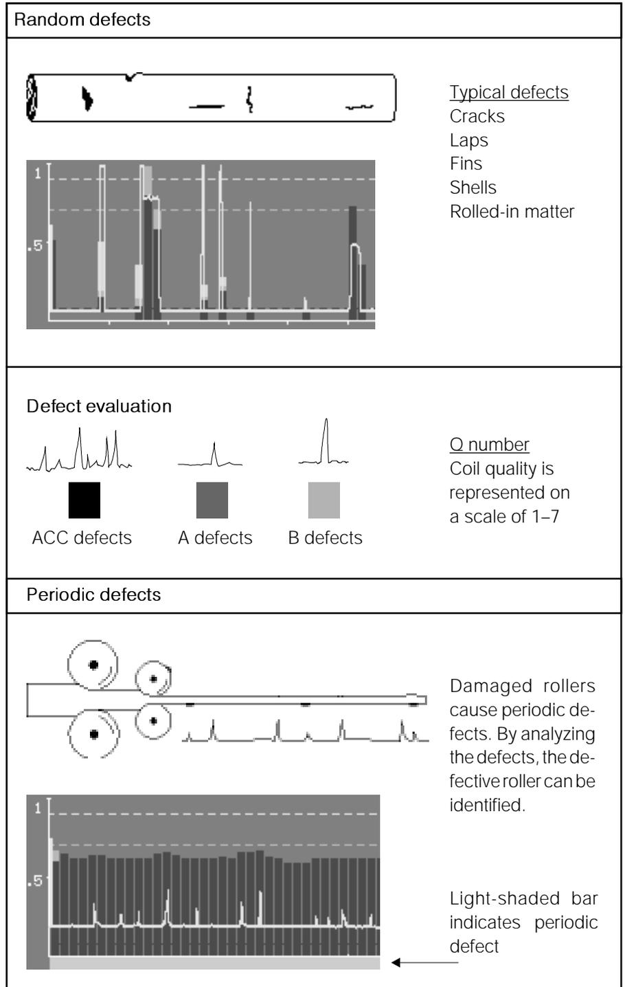
Fig. 4. Defect types
