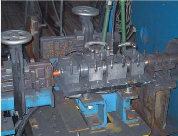
Fig. 5: Coil holder in operation with product moving left to right
