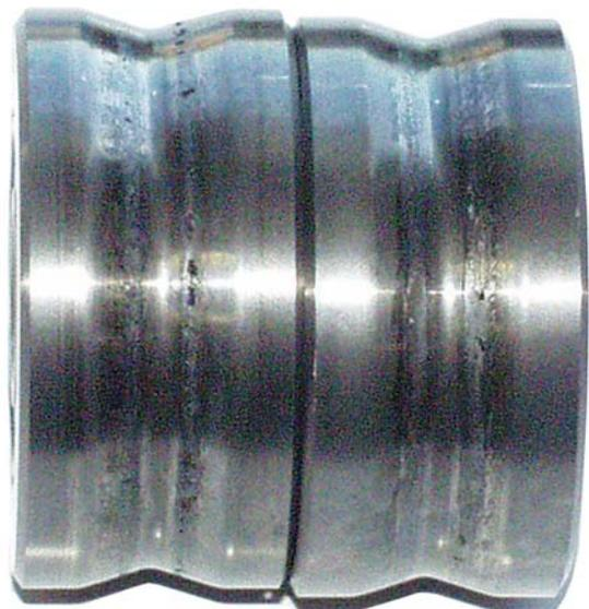
Fig. 9: Examples of worn and cracked rolls. Such defects on a roll surface lead to the typical signal sequence shown in Figure 8.
