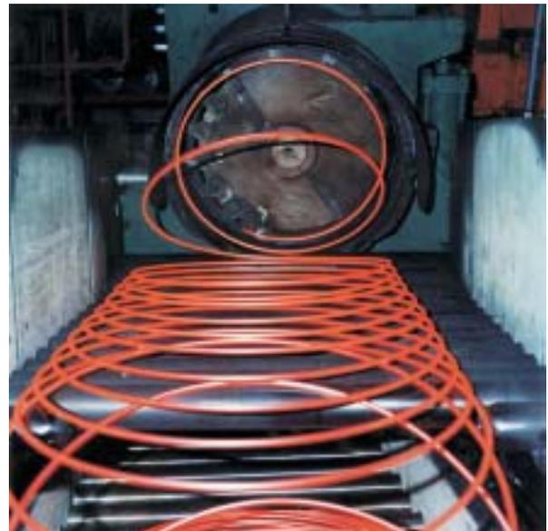
Fig. 1. Laying head in the rod mill of IWHG
