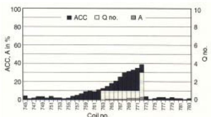
Fig 9. Increase in defects due to roll wear
