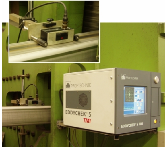
Figure 7. Testing setup in plant for square tubes showing the eddy current tester in front of the test head and the remote field probe in the insert
